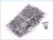
2.8mm dia x 51mm long nail fixing. Calculate 9 fixings per board to allow wastage. It is advisable to pilot hole the fixing points at the corners of boards to avoid cracking.
