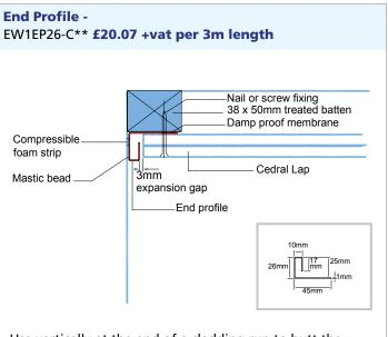
Use vertically at the end of a cladding run to butt the boards against, protecting the weatherboard and giving a straight edge framing to clad area.
