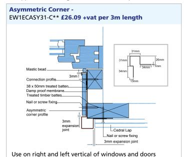
allowing for lapped boards on face side of building and single board laid flat around the reveal of window or door.
